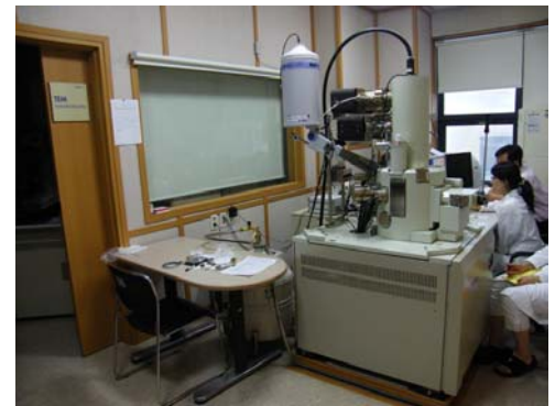
Jeol SEM JSM7401F Seoul National University, South Korea Interference from subway trains Without MagEclipse: 12 mG (0.1 - 2 Hz) With MagEclipse: 0.5 mG (0.1 - 2 Hz)
