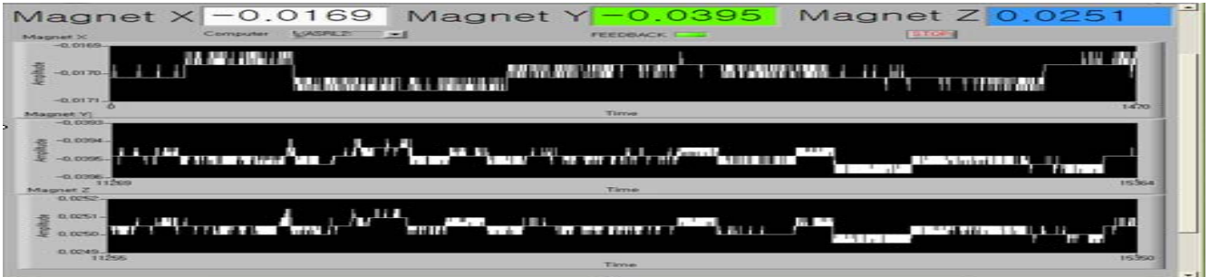
Maximum Variation value of Magnetic Field - X axis :0.2mG , Y axis : 0.3mG, Z axis : 0.3mG
