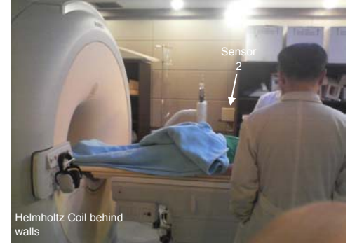
Philips 3T Jaesang Hospital, South Korea Interference from cars Without MagEclipse: 15 mG (- 1 Hz) With MagEclipse: 3 mG (- 1 Hz)
