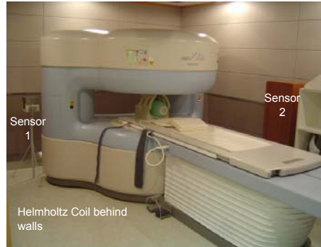
Hitachi MRI Elite 0.3T Kibyungsu Hospital, South Korea Interference from cars Without MagEclipse: 30 mG (- 1 Hz) With MagEclipse: 1 mG (- 1 Hz)
